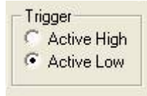
FIGURE 24. Set “Trigger” by clicking the desired option button.
